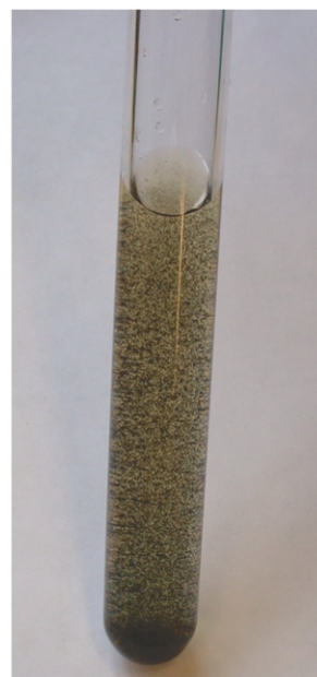
Fig. 1 Palladium metal suspension occurring in [C 4 mim][BF 4 ] upon addition of benzyl alcohol at 80 °C.
